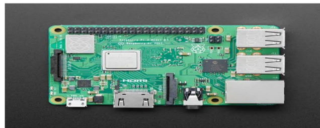
Fig 4: Raspberry Pi 3 Model B+
