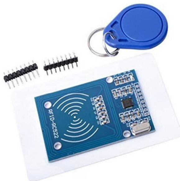
Fig 4: MiFare RFID Reader
