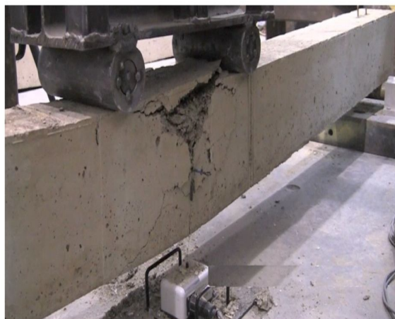
Fig.9 Fly ash/glass beam at failure [23]
