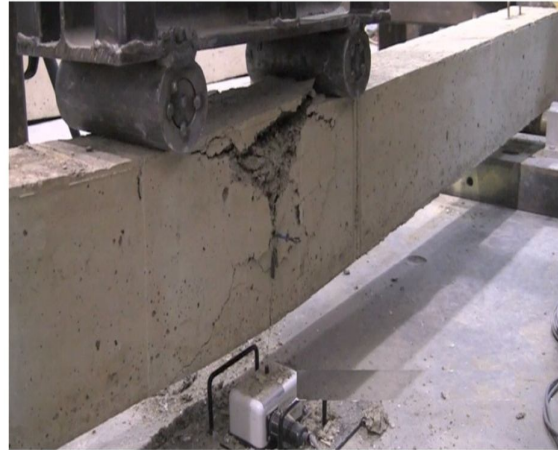
Fig.9 Fly ash/glass beam at failure [23]
