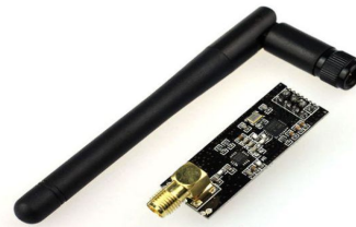
Fig 4: nRF24L01 transceiver with external antenna
