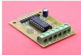
Fig.4 L293D motor driver
