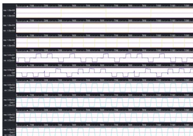
Fig. 10. Full Adder Simulation Outcomes
