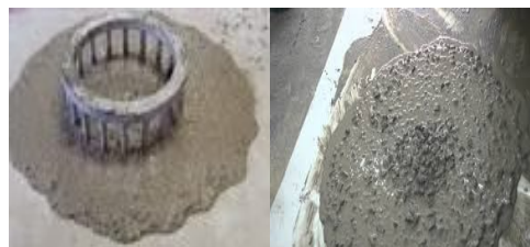
Fig-2. J-ring test
