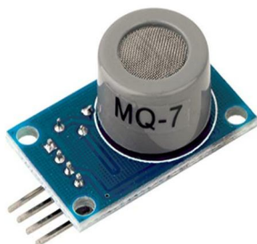
Fig 4: Carbon Monoxide Sensor
