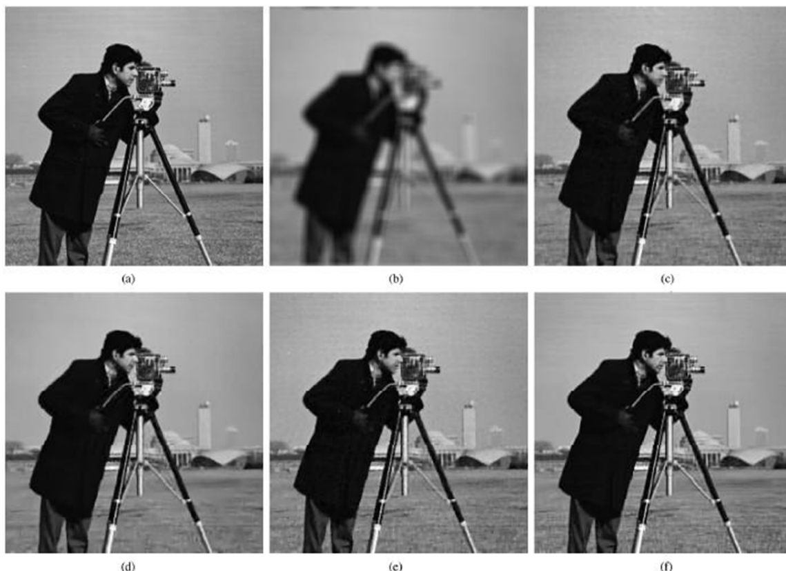
Fig. 5 comparison of original cameraman images, noisy blurred image (BSNR = 40 dB, 9 \times 9 uniform blur) and deblurred images by different algorithms); a) Original image; b) Noisy blurred image; c) TVMM (ISNR = 8.48 dB); d) SADCT (ISNR = 8.57 dB); e) IST (ISNR = 8.65 dB); f) fine-granularity and spatail-adaptive regularization (ISNR = 9.96 dB).
