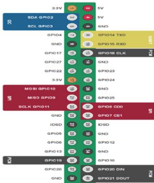
Fig.2: (a) Raspberry Pi 3 Model B (b) Pin Description of Raspberry Pi 3 [Source: Google]
