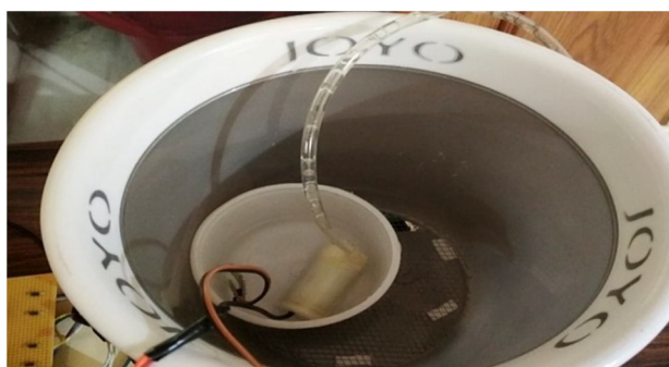
Fig 10. Water stuck in the trash detected by moisture sensor, motor turns on.
