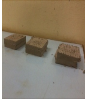
Fig. 6 Failure on Fly ash with 50% PRP
