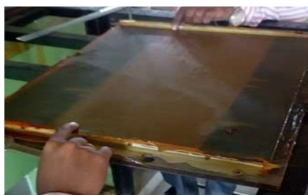
Fig 1. Composite laminate with delamination
