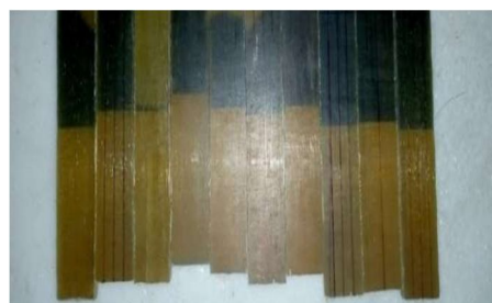
Fig 2. Specimens with delamination
