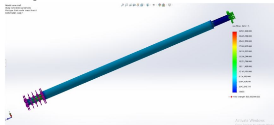
Figure 6 - Max stress (von mises)
