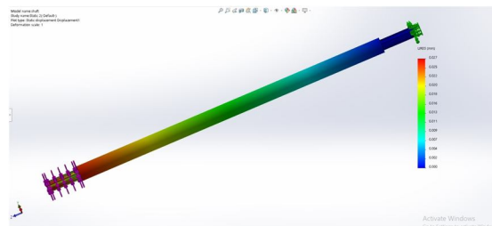
Figure 7 - Deformation (in mm)
