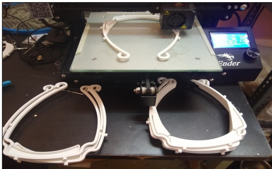
Fig.7: 3D printed frames, free source frame on left hand side and modified designed frame on left hand side.
