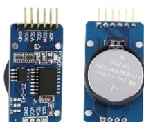
Fig. 3.2.3 Real Time Clock
