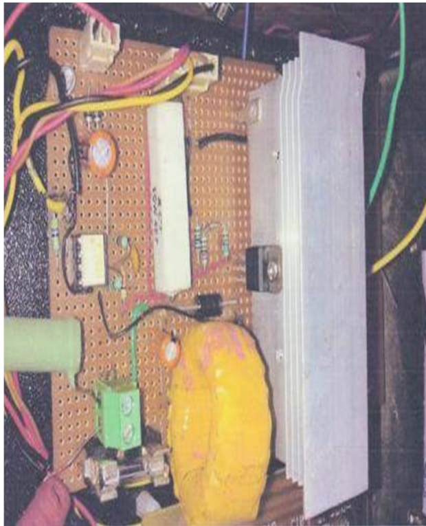
Fig. 15 Actual view of power circuit
