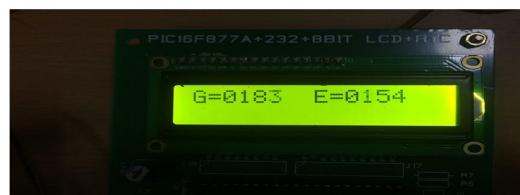
Figure 3. Output of both EEG and Gas sensor
