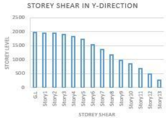
Figure 7.7 Maximum storey shear in direction of Y
