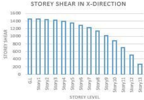
Figure 7.6 Maximum storey shear in direction of X
