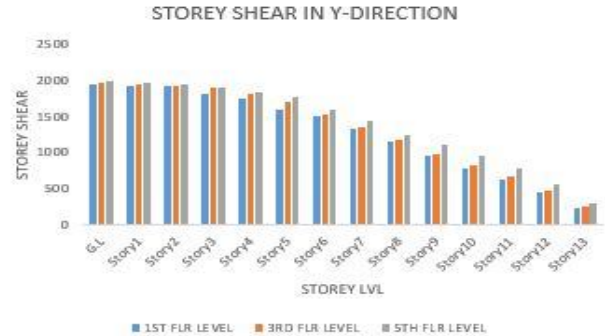
Figure 8.2 Maximum storey shear in direction of Y
