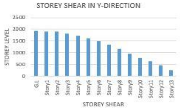
Figure 7.2 Maximum storey shear in direction of Y
