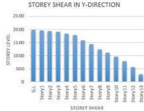
Figure 7.12 Maximum storey shear in direction of Y
