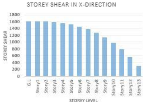
Figure 7.11 Maximum storey shear in direction of X
