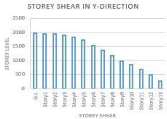
Figure 7.7 Maximum storey shear in direction of Y
