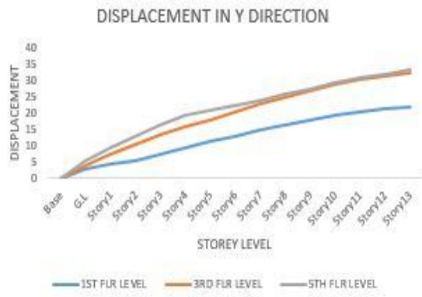
Figure 8.4 Joint displacement in direction of Y
