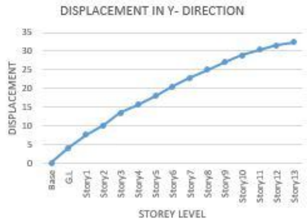
Figure 7.9 Joint displacement in direction of Y
