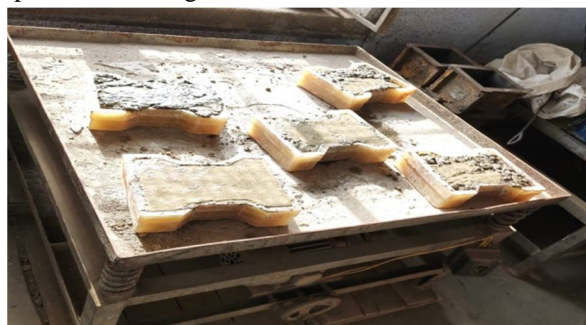
Figure 3: Casting of paver block
