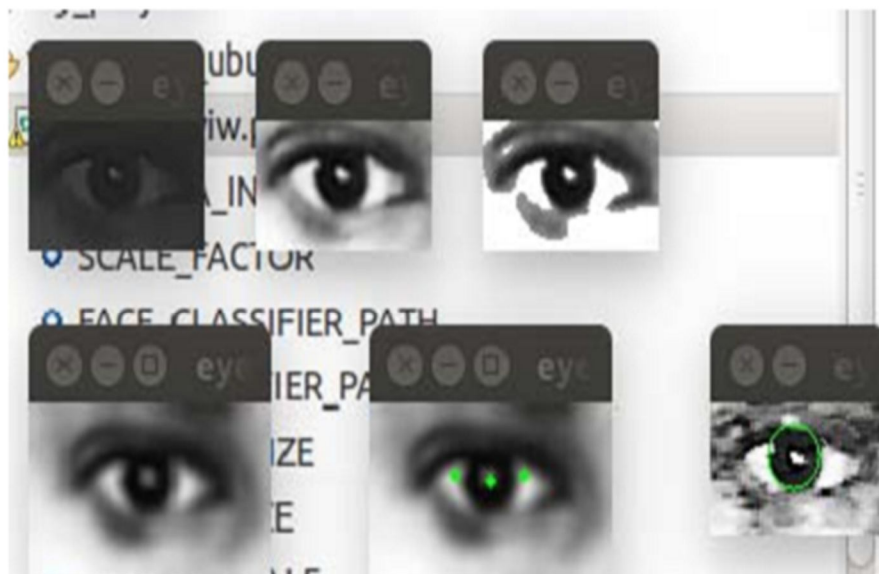
Fig 2.7 Obtained eye center and detected circle
