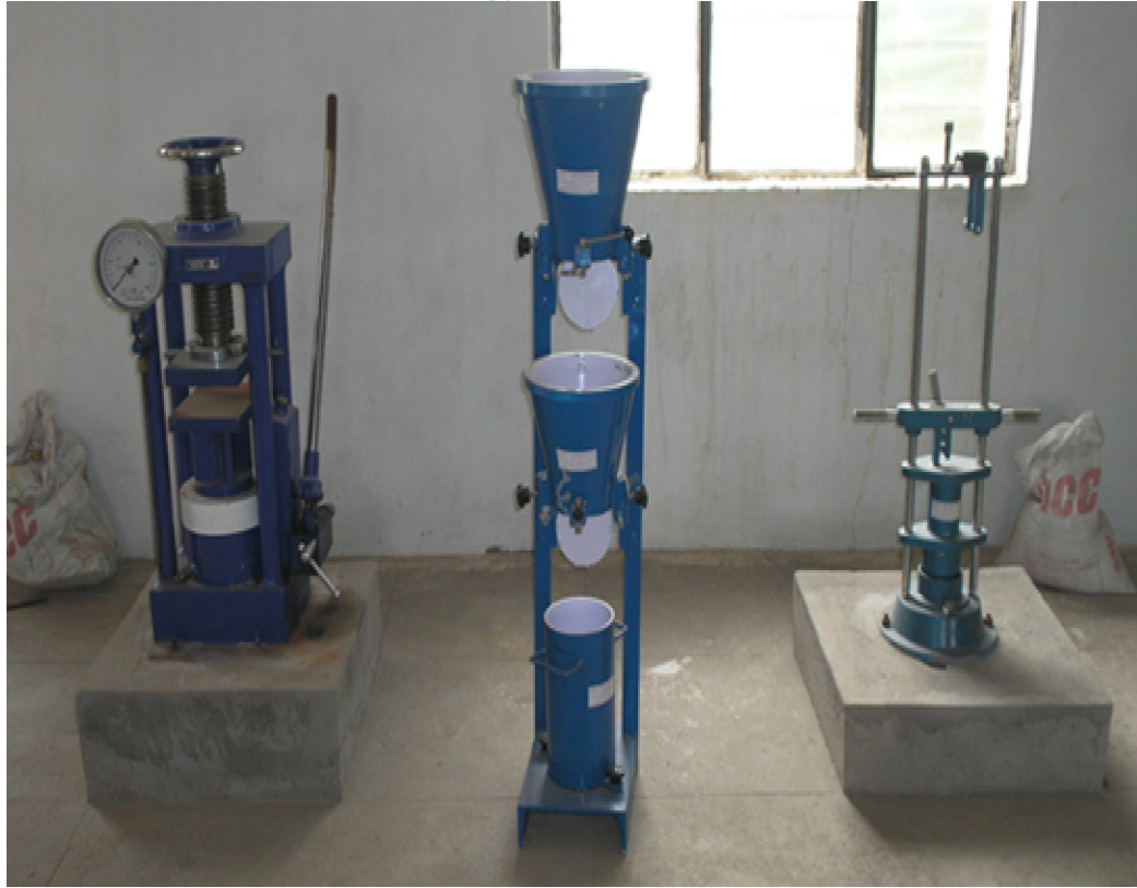
Fig 3.2 Compaction Factor Test
