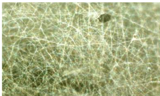
Fig 2(a) Optical microscope image of PVA Composites
