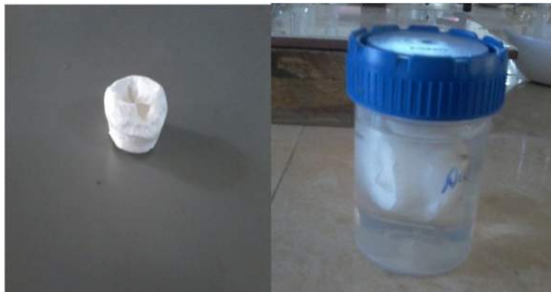
Fig 3 (a) Foam formed using TIPS technique
