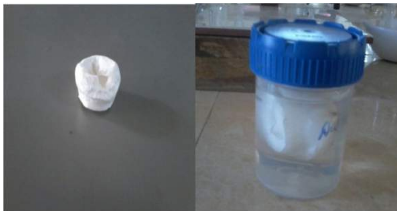
Fig 3 (a) Foam formed using TIPS technique
