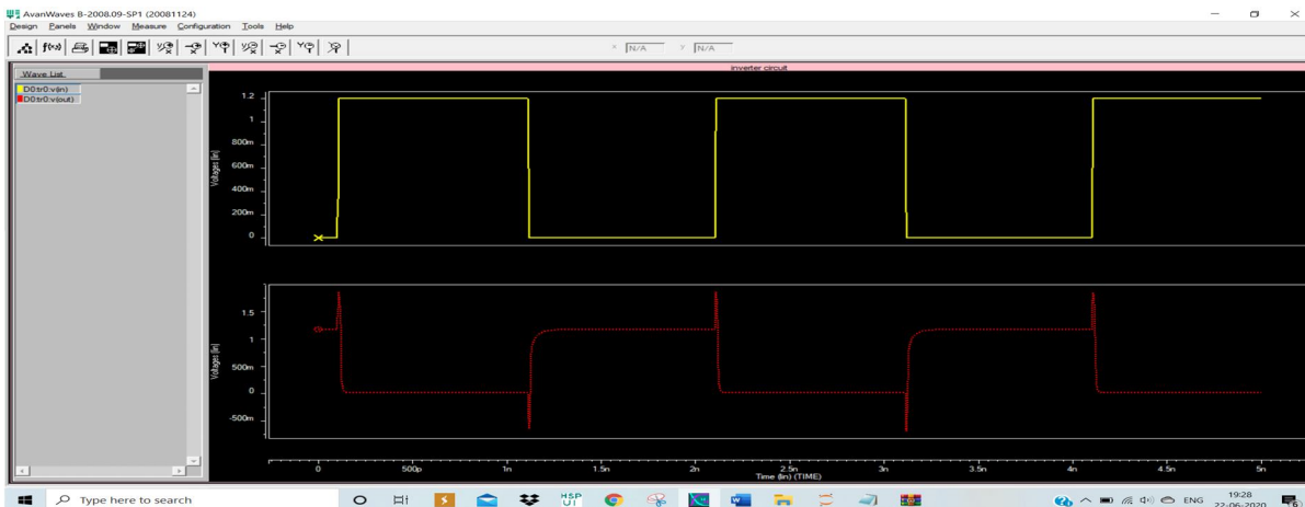
Fig (m) Simulations results Inverter logic of CMOS PTM model Inverter
