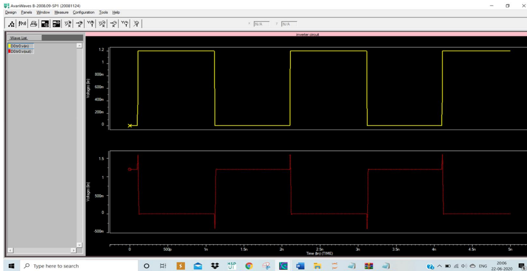
Fig (n) Simulations results Inverter logic of CMOS TSMC model Inverter
