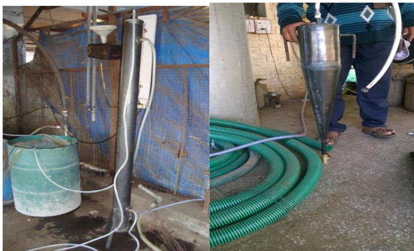
Fig 1 Water Scrubbing Unit Fig 2 Cyclone Scrubbing Unit
