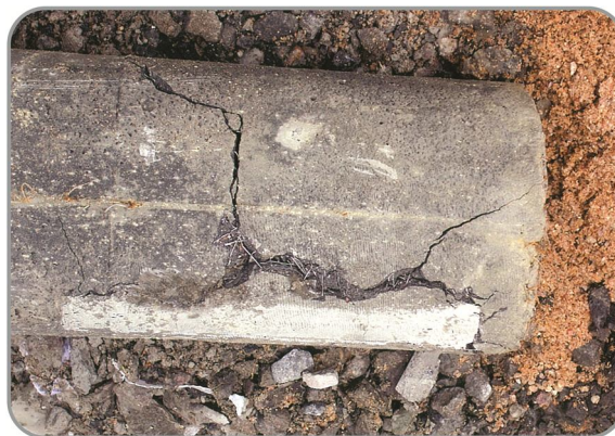
Fig. 5 UHPFRC Specimen after Testing
