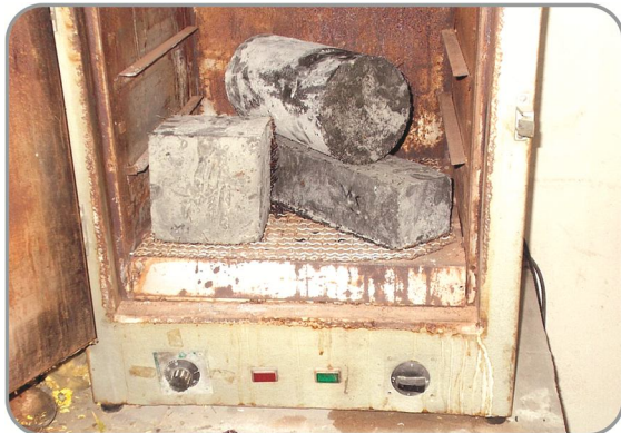
Fig. 3 UHPFRC Hot Air Curing
