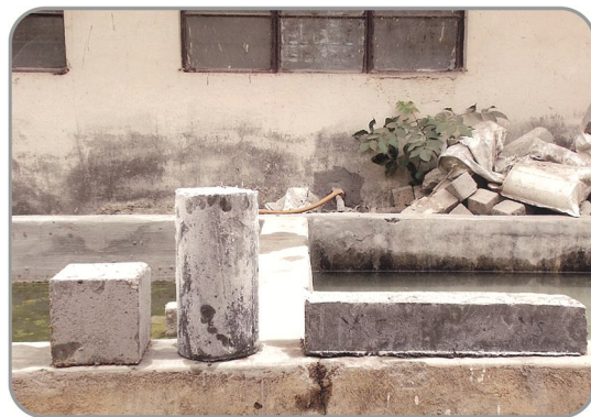
Fig. 2 Specimens after Curing
