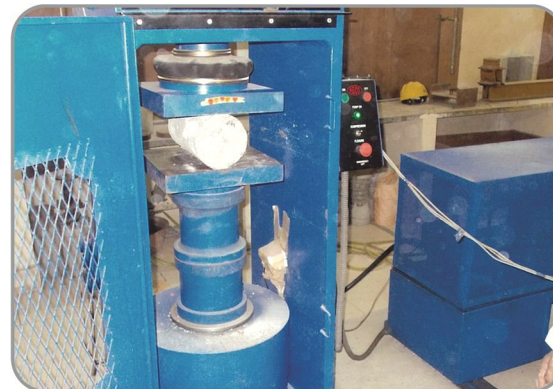
Fig. 4 Test Setup Tensile Automatic CTM (3000 KN)
