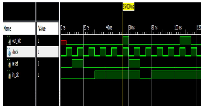
Figure 11: Simulation Result of the Sequence Detector.
