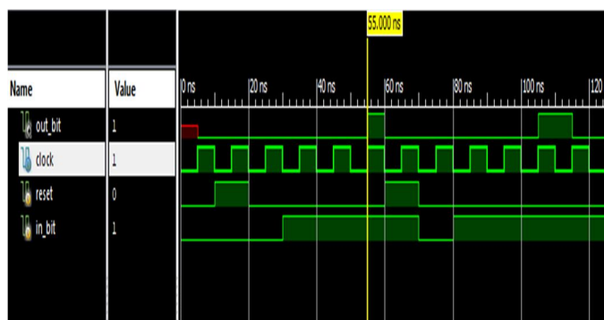
Figure 11: Simulation Result of the Sequence Detector.
