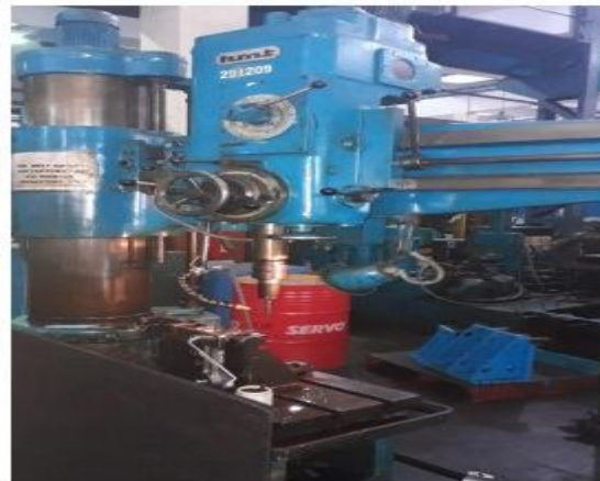
Fig 8. Mounting of Jigs and fixture on Radial Drilling machine
