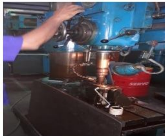
Fig 9. Machining of connecting rod on Jigs and fixture in Radial drilling machine
