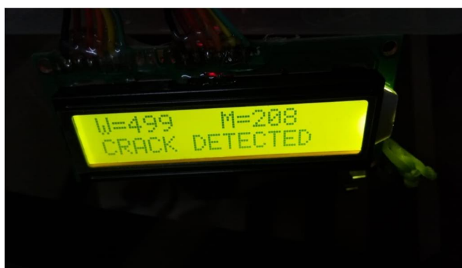
Fig. 10. LCD shows the message crack detected.
