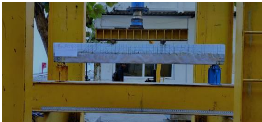
Fig 12. Failure pattern of BWRC 40.
