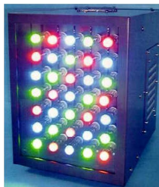
Fig. 13 CNT field emission lamps arrayed in a 5-by-7 matrix
