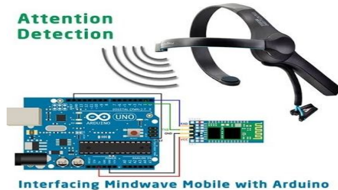
Fig. 4. Neurosky Mind Wave Headset
