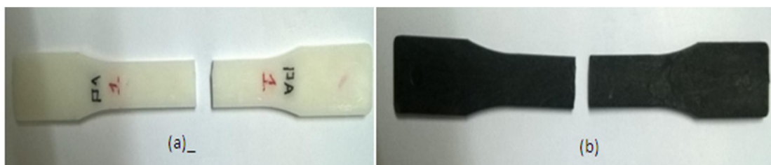
Figure 7: (a) Specimen after tensile test pure acetal (b) Specimen after tensile test pure acetal
