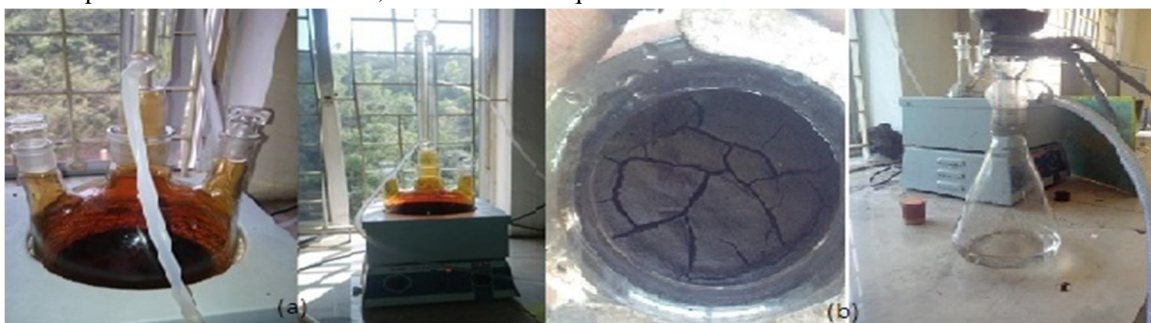
Figure 2: (a) Refluxing Setup (b) Filtration Setup
