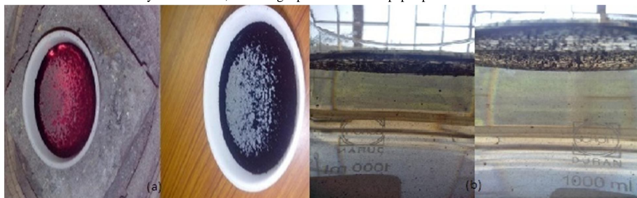
Figure1: (a) After Calcinations Impurities formed on the Top (b) Impurities Floating on the Top
