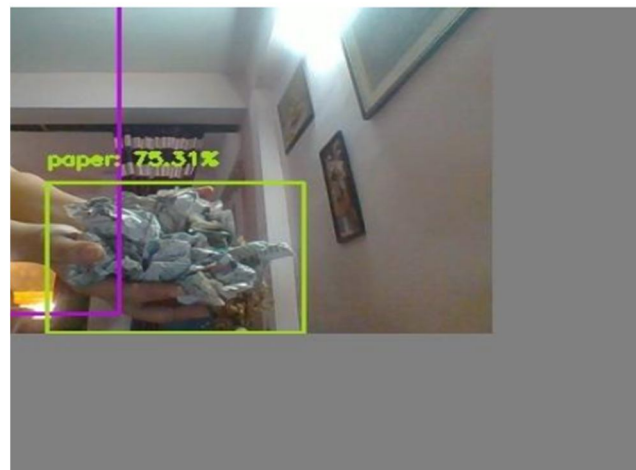
Fig-8 Paper Detection using Caffe Model
