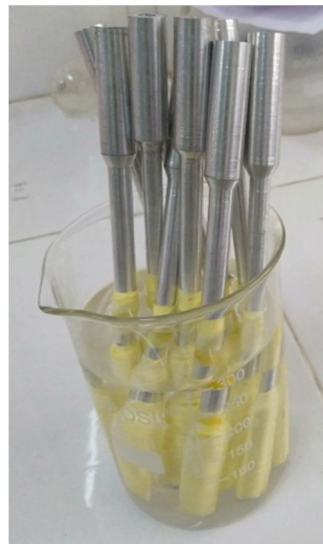
Fig 7: Specimens dipped in salt solution
