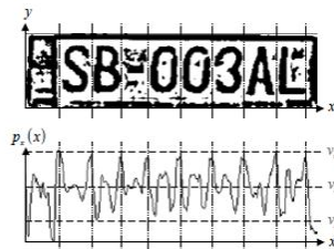
Fig. 10 a) number plate after application of the adaptive thresholding, b) horizontal projection of plate with detected peaks
