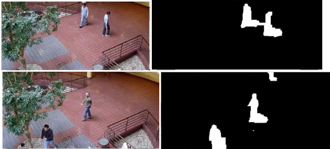
Fig. 3 Background subtraction using LSD
