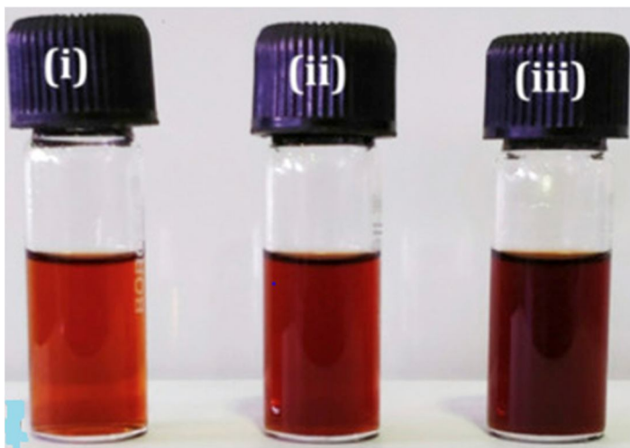
Figure 6 Combination of dye 1) 15ml Red + 15ml Green, 2) 10ml Red +20ml Green, 3) 20 Red + 10ml Green
