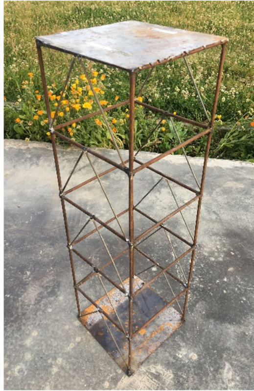
Fig A.29 Inverted V steel frame model
