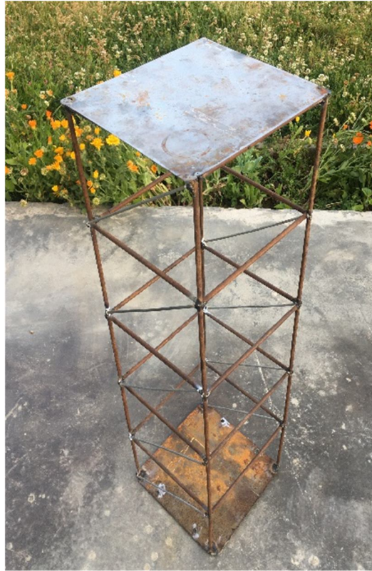
Fig A.27 Diagonal steel frame model
