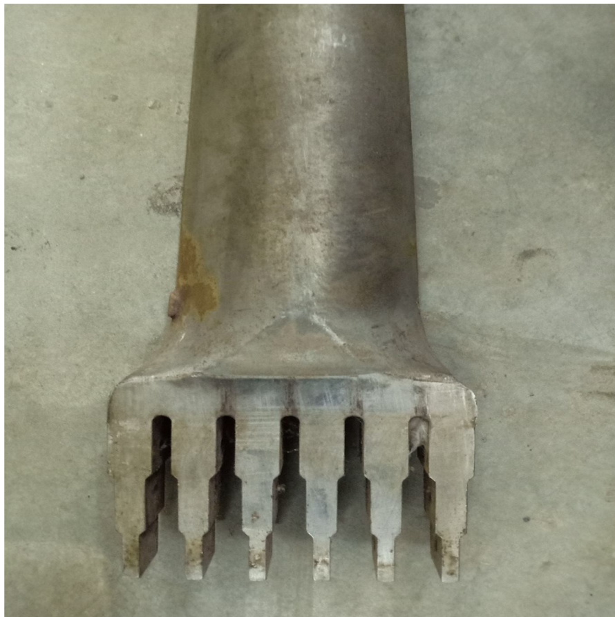
Fig. 4 Multi Fork / Finger type root attachment
