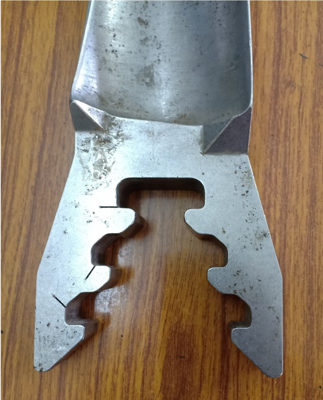
Fig. 5 Straddle type root attachment
