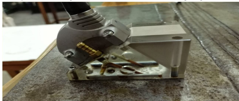
Fig. 10 PAUT Probe with Wedge
