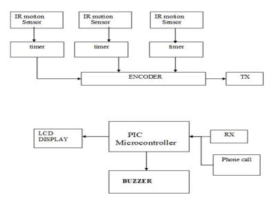
Fig.1- Block Diagram of Shop Security System Using Radio Frequency Wave
