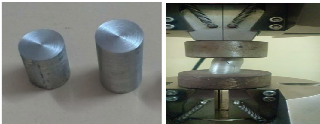
Fig 1.2 and 1.3 Machined Samples and compression test on UTM
