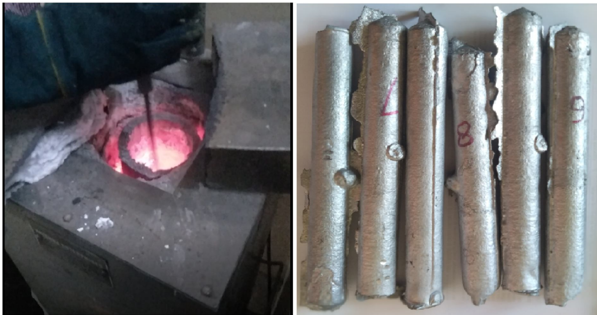
Fig 1.1 stir casting set up and Fabricated Cylindrical samples
