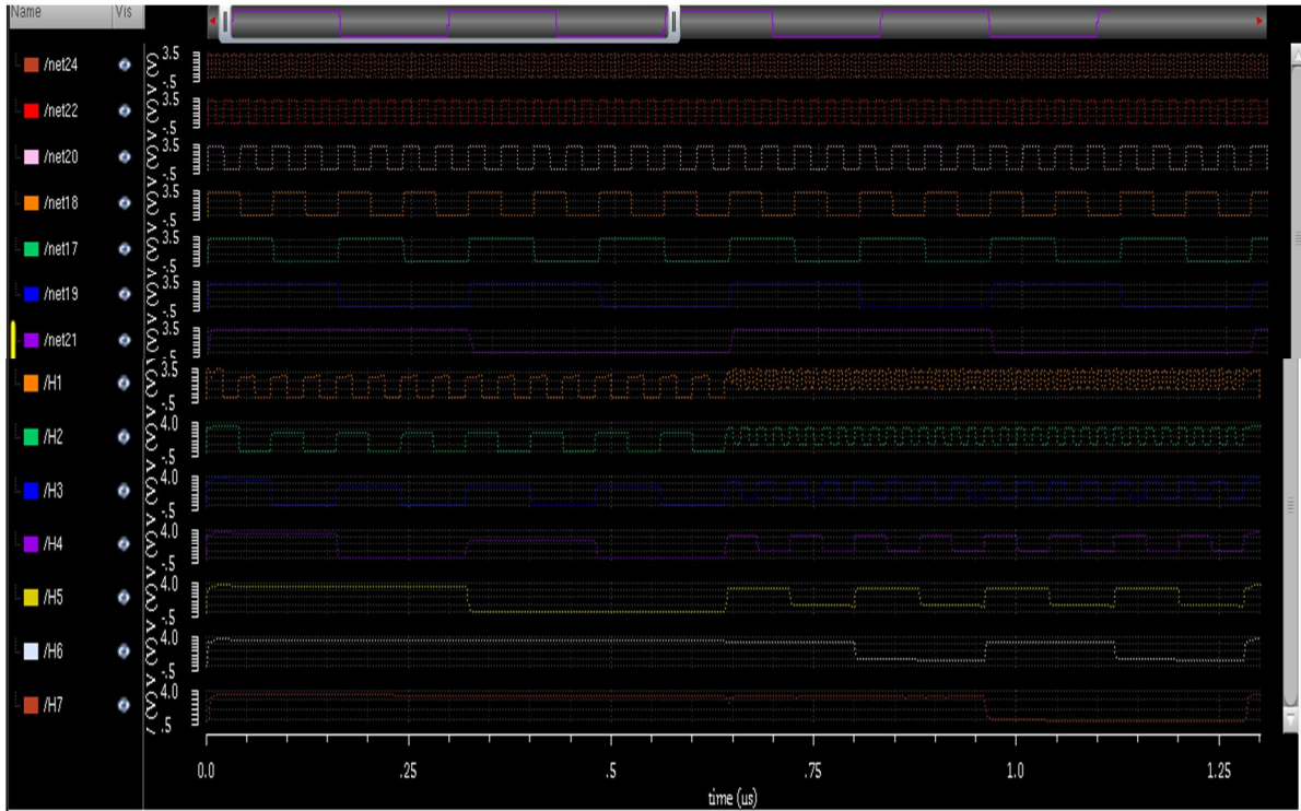
Fig 35:8-Bit Shift left/right output waveform
