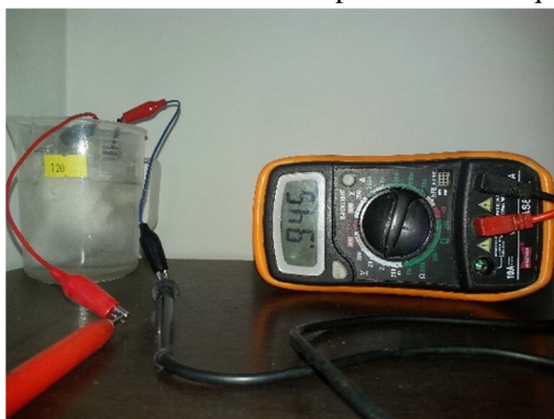
Fig. 3: The battery generating up to 1 V
