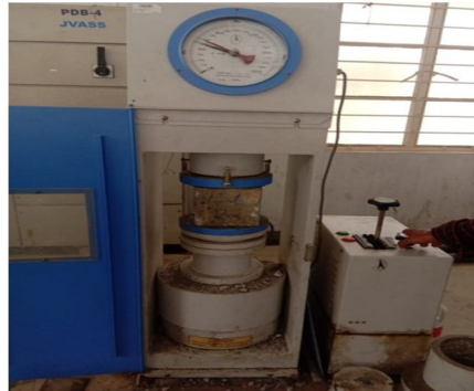
Fig 6: Testing of cubes
