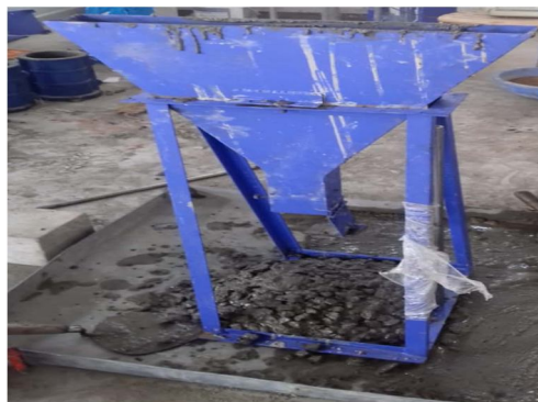
Fig 5: V Funnel Test
