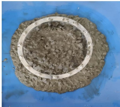
Fig 4: J Ring Test
