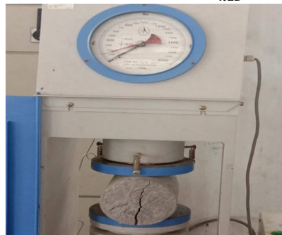
Fig 7: Testing of cylinder
