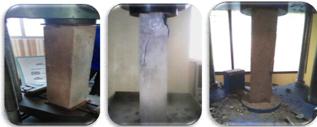
Fig 5.3 During Testing and failure pattern of Ultimate load carrying capacity of Columns
