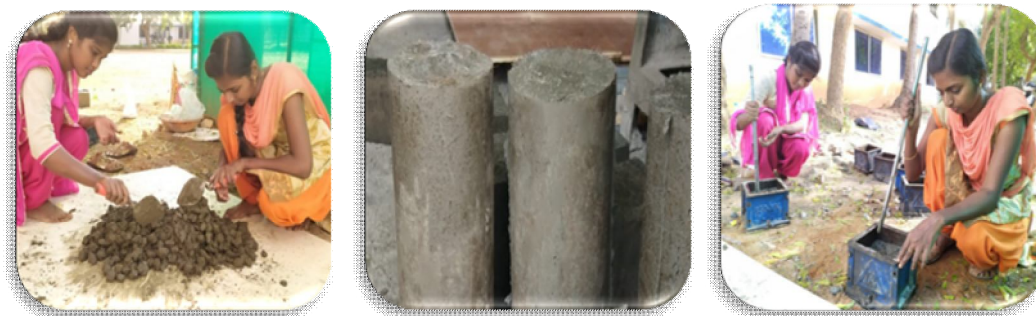
Fig 4.1 Mixing of Concrete ingredients and Casting of specimen
