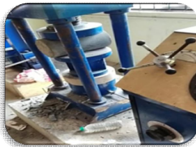
Fig 5.2 During Testing of Splitting tensile strength of cylinder
