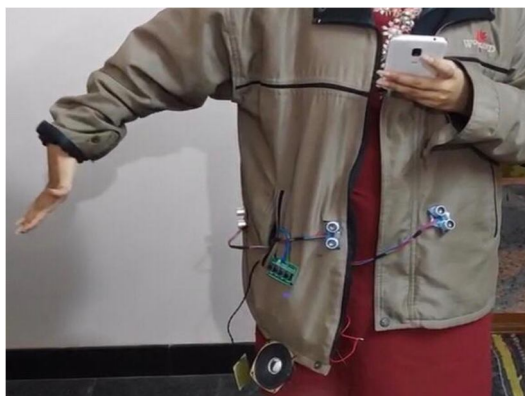
Fig 4: Obstacle detection on the right side
