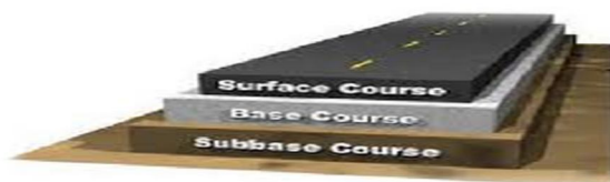
Fig 1: Different layers of Road
