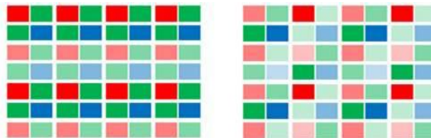
Fig. 6 Spatially Varying Exposure using 2 lines and Spatially Varying Exposure using different pixel exposures
