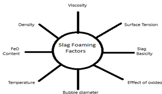
Fig. 2 Factors related to slag foaming
