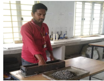
Fig: Preparation and casting of test specimens
