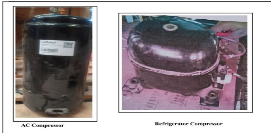
Fig. 3: AC Compressor and Domestic Refrigerator Compressor
